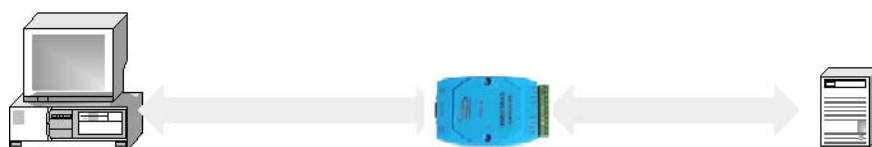
计算机-----CAN232MB/CAN485MB-----CAN设备
